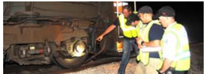
WTLC General Superintendent Matt Jackson demonstrates the operation of shelf couplers. The safety couplers are required on HazMat tank cars.
