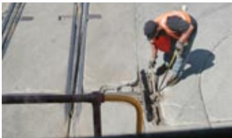
Kyle Kimpel, conductor, operates an in-ground switch, which is hidden by an iron panel and lays flat on the street, when not in use.
